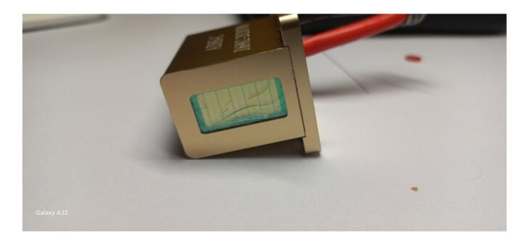
One of the typical problems of the diode laser is that the laser does not emit flash and does not cause sensations. Damage can be detected visually through the transparent part of the handle.
