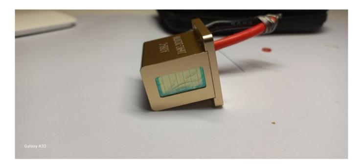
The most common problem with the diode laser handle - the laser stops issuing impulses, there are no sensations. Through the observation window, the cause of the breakdown is often visible.
