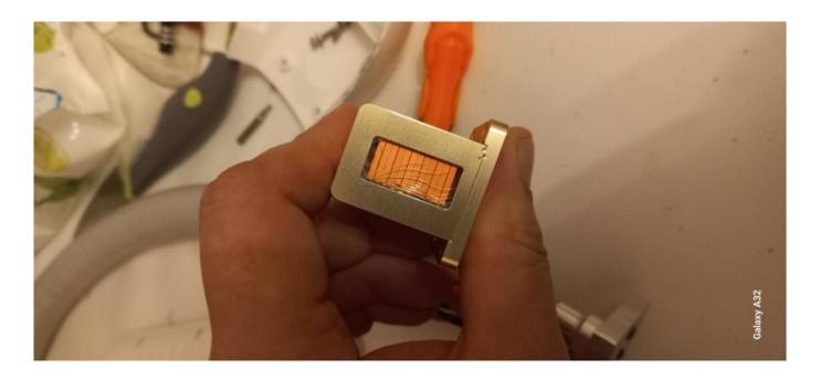
The most common problem with the diode laser handle is not visible light impulses, there is no contact with the skin. Damage is often visible through the observation glass.
