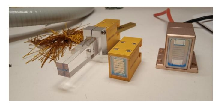
One of the typical problems of the diode laser is that the laser does not emit flash and does not cause sensations. The handle defect is often visually observed through the window.
