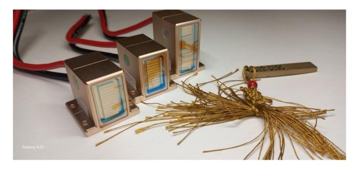
The main defect in the work of the diode handle is that light impulses are not visible, there is no contact with the skin.Often it is enough to look out the window of the pen to see the problem.
