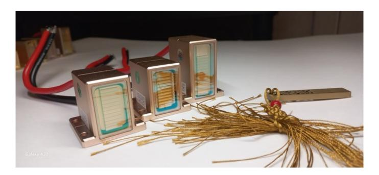
Often, the diode laser has a problem: the flashes stop and the sensation of tingling disappears. Damage can be detected visually through the transparent part of the handle.
