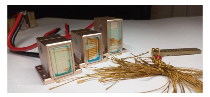
The main defect in the work of the diode handle is that the laser stops issuing impulses, there are no sensations.Damage is often visible through the observation glass.
