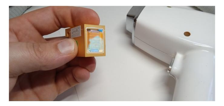
In most cases, the handle malfunction is due to the fact that there is a loss of flashes and sensations. Through the observation window, the cause of the breakdown is often visible.
