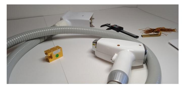
Often, the diode laser handle fails: there is a loss of flashes and sensations.Damage is often visible through the observation glass.
