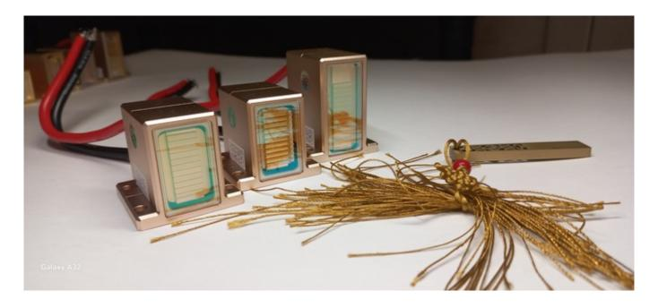
Often, the diode laser handle fails: no light impulses are visible, there is no contact with the skin.Damage can be detected visually through the transparent part of the handle.
