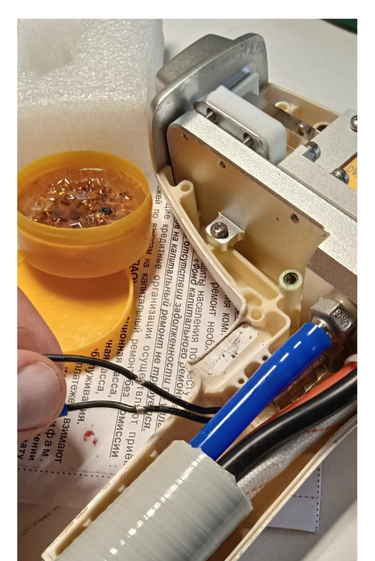
In most cases, the handle malfunction is due to the fact that the impulses do not pass, the patient does not feel tingling. Often the problem is determined visually through the window on the handle.
