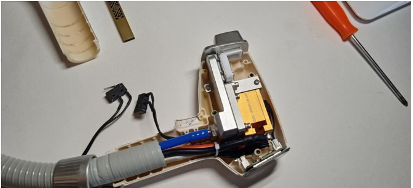
Issues in the work of the diode laser handle are expressed as follows: the laser does not work, and the sensations disappear. When examining through the window, you can notice a malfunction.
