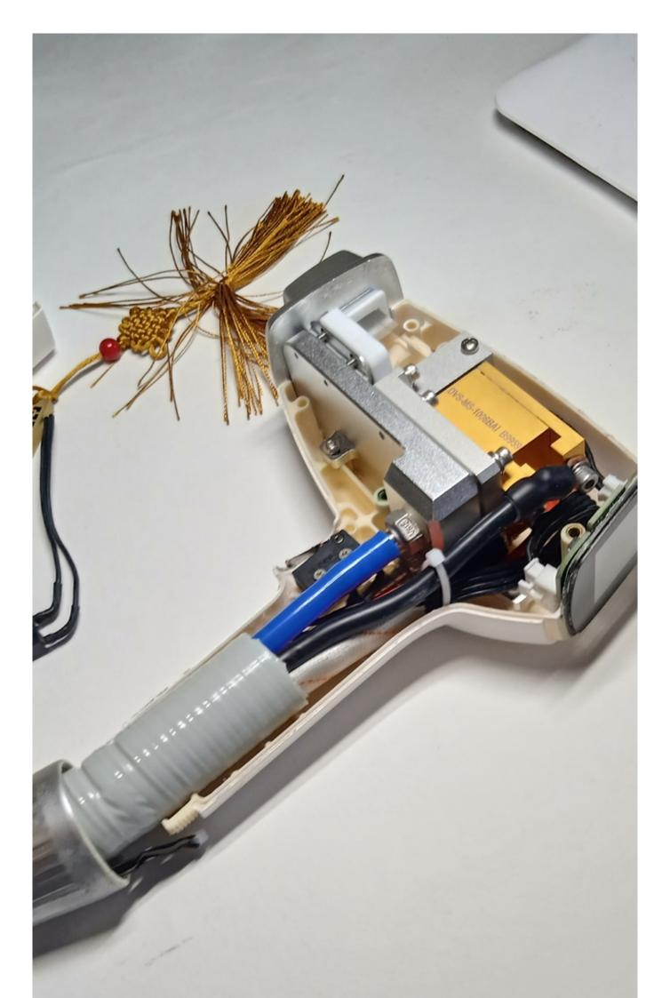
Frequent malfunction of the laser handle - the laser stops issuing impulses, there are no sensations. Damage can be detected visually through the transparent part of the handle.
