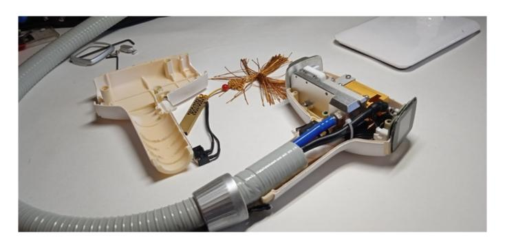
Often, the diode laser handle fails: there is a loss of flashes and sensations. The breakdown is often noticeable when examining the handle.
