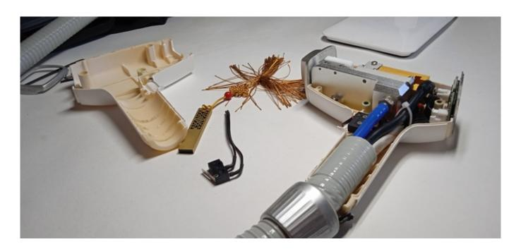
The most common problem with the diode laser handle is not visible light impulses, there is no contact with the skin. Often the problem is determined visually through the window on the handle.
