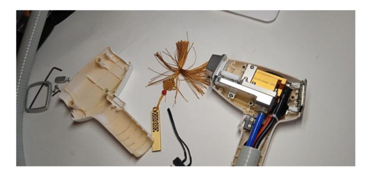
The most common problem with the diode laser handle - there is a loss of flashes and sensations. Damage can be detected visually through the transparent part of the handle.
