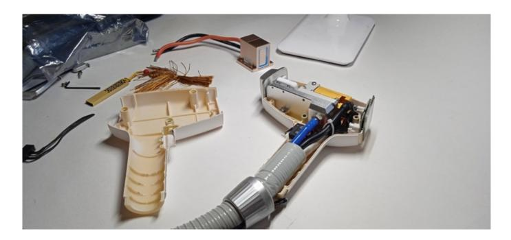
Frequent malfunction of the laser handle - there are no visual flashes and sensations on the skin. The breakdown is often noticeable when examining the handle.
