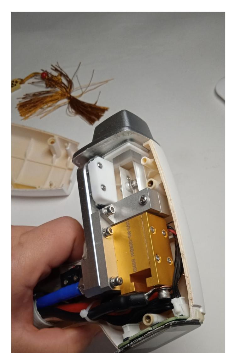
The malfunctions of the diode laser handle are expressed in the following: no light impulses are visible, there is no contact with the skin.Damage is often visible through the observation glass.
