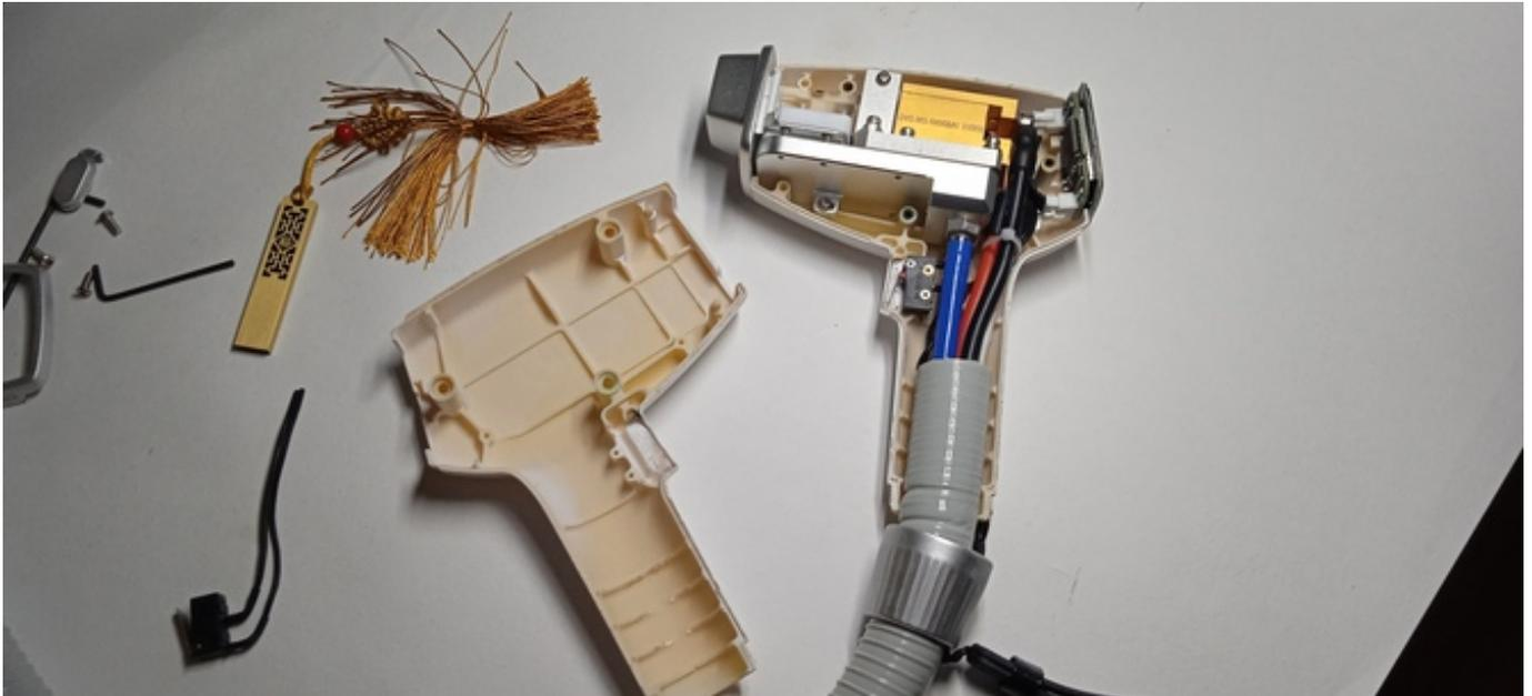
A common breakdown of the handle is that the outbreaks stop and the sensation of tingling disappears. Often the problem is determined visually through the window on the handle.
