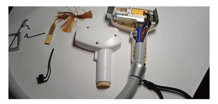
The main reason for the breakdown of the diode laser handle is that flashes disappear and there is no tingling. Often the problem can be seen through the observation window.
