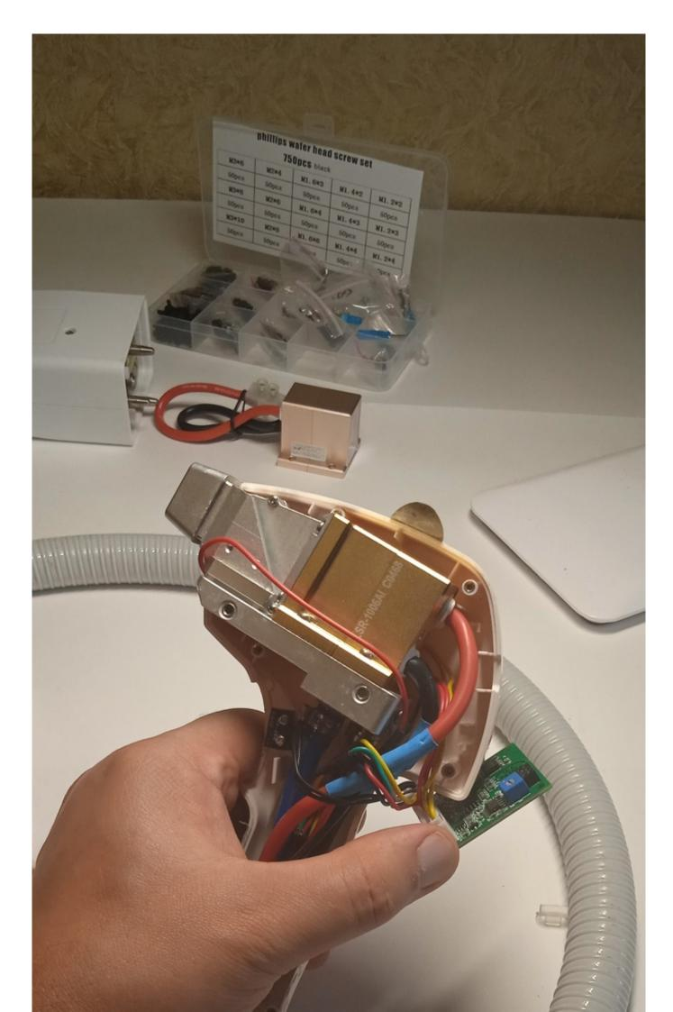
Dithes in the work of the diode laser handle are expressed as follows: the laser does not work, and the sensations disappear. The handle defect is often visually observed through the window.
