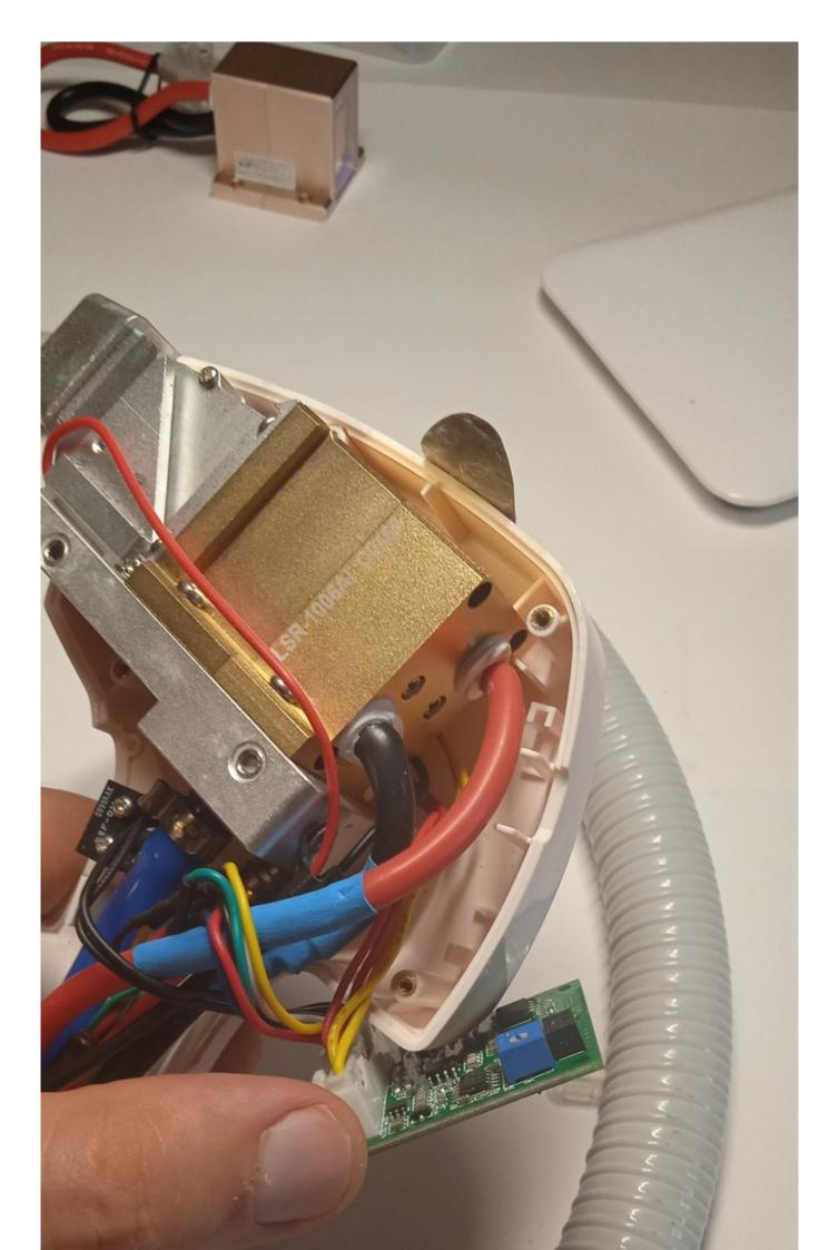
Often, the diode laser has a problem: there are no light impulses, there is no contact with the skin. Damage is often visible through the observation glass.
