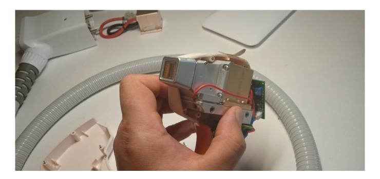
Often, the diode laser has a problem: the laser stops issuing impulses, there are no sensations. The breakdown is often noticeable when examining the handle.
