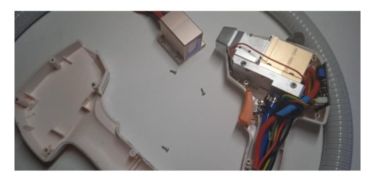
Often, the diode laser handle fails: the laser ceases to give out impulses, there are no sensations. Damage is often visible through the observation glass.
