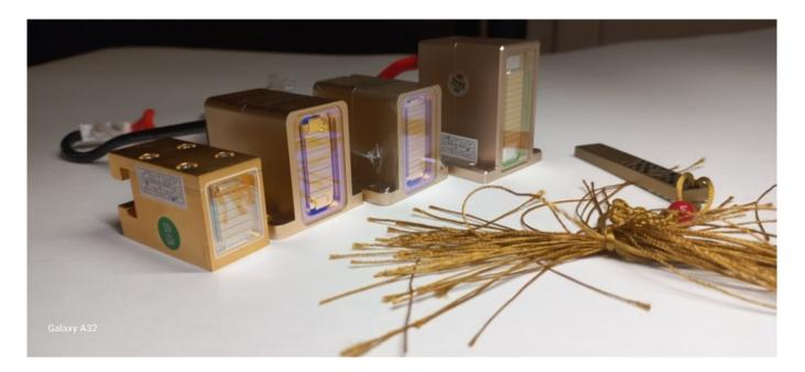
A common breakdown of the handle is that there is a loss of flashes and sensations.Damage can be detected visually through the transparent part of the handle.
