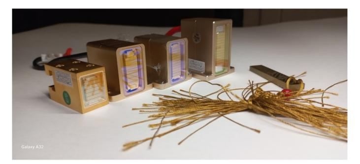
The malfunctions of the diode laser handle are expressed in the following: no light impulses are visible, there is no contact with the skin.Often the problem is determined visually through the window on the handle.
