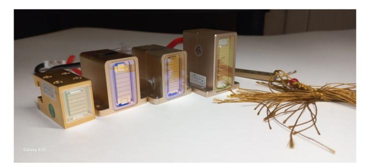
The most common problem with the diode laser handle - the laser stops issuing impulses, there are no sensations. Often the problem can be seen through the observation window.
