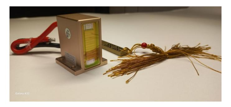
Frequent failure of the laser handle - the laser does not work, and the sensations disappear. Sometimes it can be recognized visually by looking out the window.
