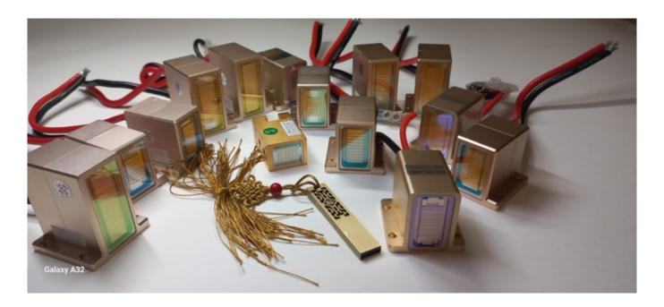
Often, the diode laser has a problem: there is a loss of flashes and sensations. The handle defect is often visually observed through the window.
