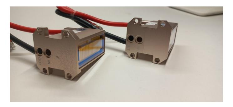
The main reason for the breakdown of the diode laser handle is the laser does not work, and the sensations disappear. Damage is often visible through the observation glass.
