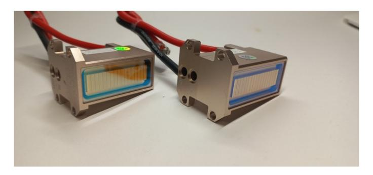
Frequent fault of the laser handle - flashes disappear and there is no tingling. Often the problem is determined visually through the window on the handle.
