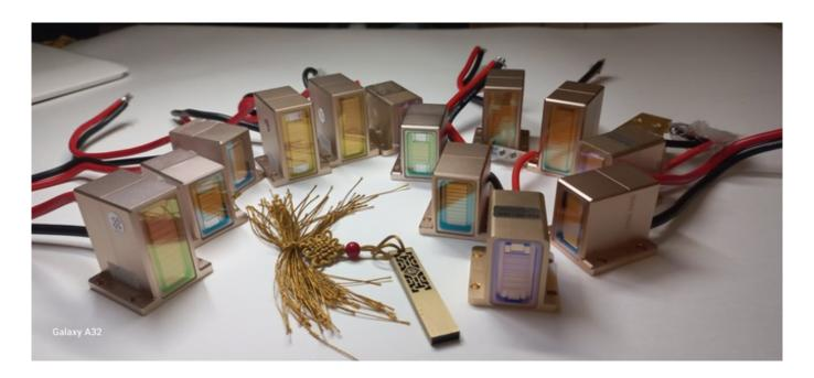
Dithes in the work of the diode laser handle are expressed as follows: the laser stops issuing impulses, there are no sensations. The handle defect is often visually observed through the window.
