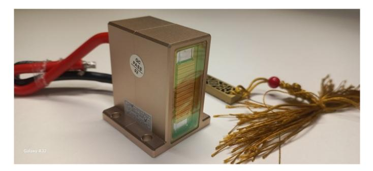
The main reason for the breakdown of the diode laser handle is the flashes stop and the sensation of tingling disappears. Often the problem can be seen through the observation window.
