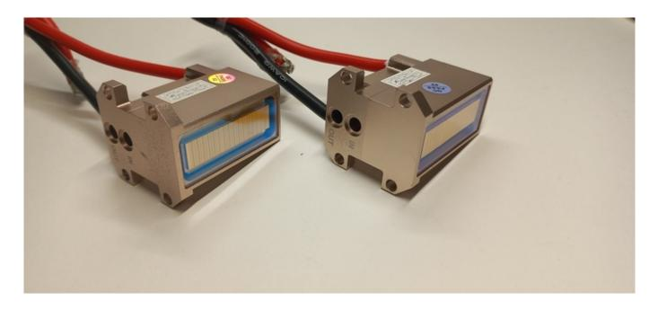
Often, the diode laser has a problem: the laser does not emit flash and does not cause sensations. Often the problem can be seen through the observation window.
