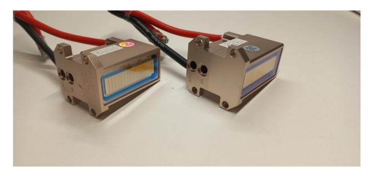
The most common problem with the diode laser handle - the laser stops issuing impulses, there are no sensations. Often it is enough to look out the window of the pen to see the problem.
