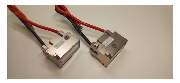
A common breakdown of the handle is that there is a loss of flashes and sensations. Often the problem can be seen through the observation window.
