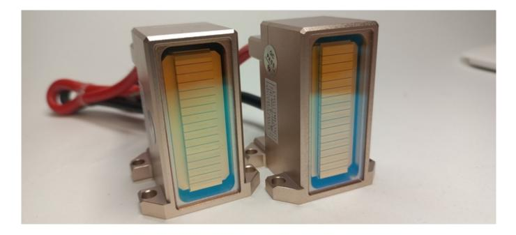
The most common problem with the diode laser handle is the laser does not work, and the sensations disappear. The handle defect is often visually observed through the window.
