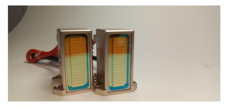
The most common problem with the diode laser handle - there is a loss of flashes and sensations. The handle defect is often visually observed through the window.
