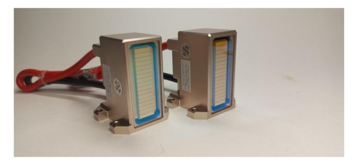
The main defect in the work of the diode handle is that the laser stops issuing impulses, there are no sensations. Often the problem can be seen through the observation window.
