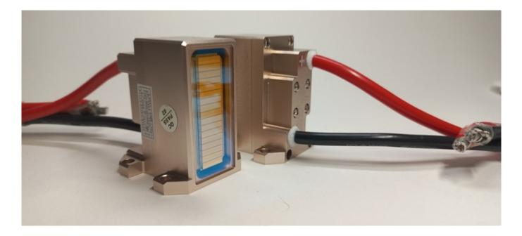
Often, the diode laser handle fails: no light impulses are visible, there is no contact with the skin.Often the problem is determined visually through the window on the handle.
