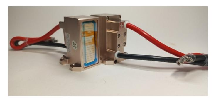
Often, the diode laser has a problem: flashes do not occur, there is no tingling either. Damage can be detected visually through the transparent part of the handle.
