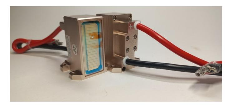
Often, the diode laser handle fails: the impulses do not pass, the patient does not feel tingling. Damage can be detected visually through the transparent part of the handle.
