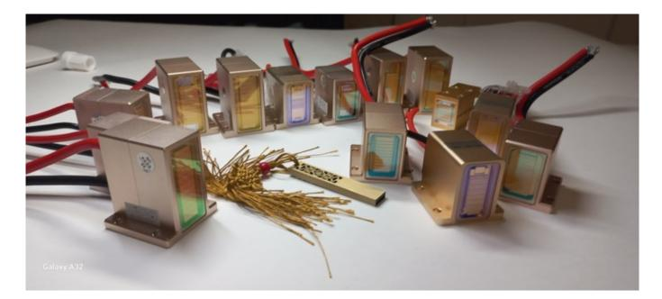
The most common problem with the diode laser handle is the laser does not emit flash and does not cause sensations. The handle defect is often visually observed through the window.
