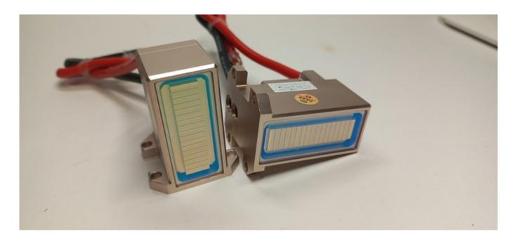
Often, the diode laser handle fails: no light impulses are visible, there is no contact with the skin. The breakdown is often noticeable when examining the handle.
