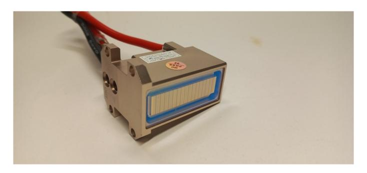
Often, the diode laser has a problem: the flashes stop and the sensation of tingling disappears. Through the observation window, the cause of the breakdown is often visible.
