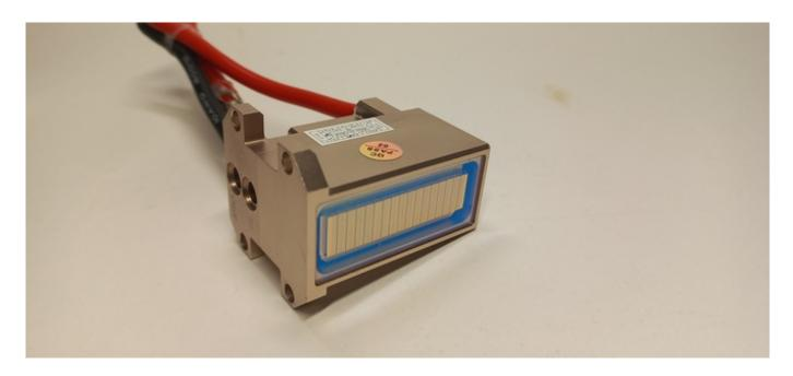
In most cases, the handle malfunction is due to the fact that light pulses are not visible, there is no contact with the skin. The handle defect is often visually observed through the window.
