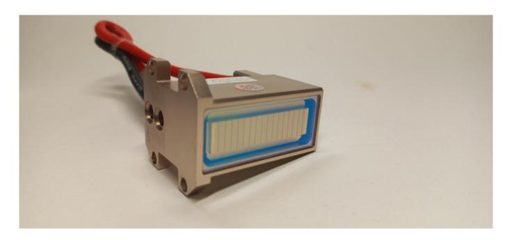
The most common problem with the diode laser handle - impulses do not pass, the patient does not feel tingling. Often the problem can be seen through the observation window.
