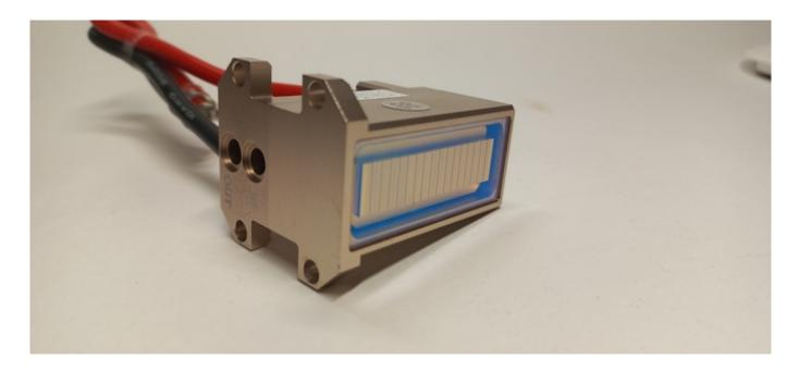
The most common problem with the diode laser handle - the flashes stop and the sensation of tingling disappears.Damage can be detected visually through the transparent part of the handle.
