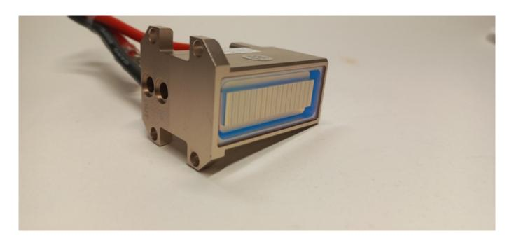
In most cases, the handle malfunction is due to the fact that the laser does not emit flash and does not cause sensations. Damage is often visible through the observation glass.
