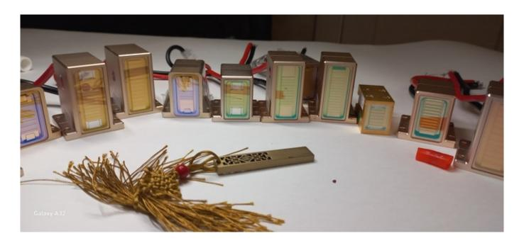
Often, the diode laser handle fails: the laser does not work, and the sensations disappear. The handle defect is often visually observed through the window.
